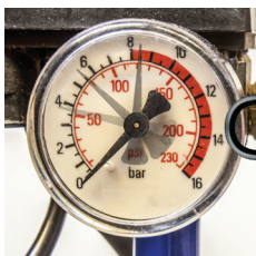
Air pressure increased to compensate for low weld force
